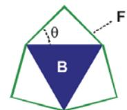
*Figure 1 An example of a basic element used for making the structures described here. In this case the block, B, is triangular and the frame, F is hexagonal. The angle  $\theta$  is critical.*
